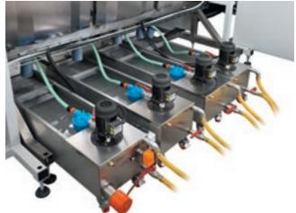
The tanks are mounted on wheels to facilitate movement during the cleaning phase. The water inside the tanks passes through two different stages of filtration before being recirculated inside the machine. The tank of the first pair of brushes contains a heating element and a thermostat for water heating. The option of heating the water in the other tanks facilitates the removal of residues and helps to dry the glass sheets. (optional).
