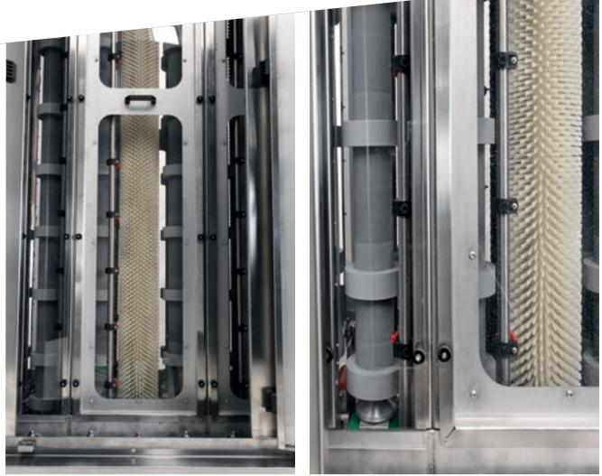
A targeted jet of water is directed towards the glass during the washing and rinsing phases, courtesy of bars fitted with special nozzles that guarantee perfect coverage of the entire sheet of glass.
