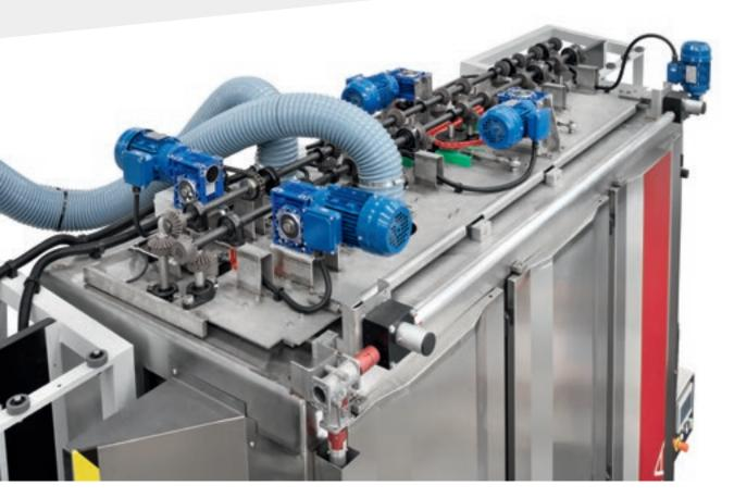
The roller and brush transmission system are positioned on the upper part of the machine for improved protection against water, and to enable facilitated inspection and maintenance.
